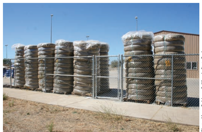
These certified weed-free rice straw wattles are contained in plastic packaging to protect them from invasive plant establishment.
